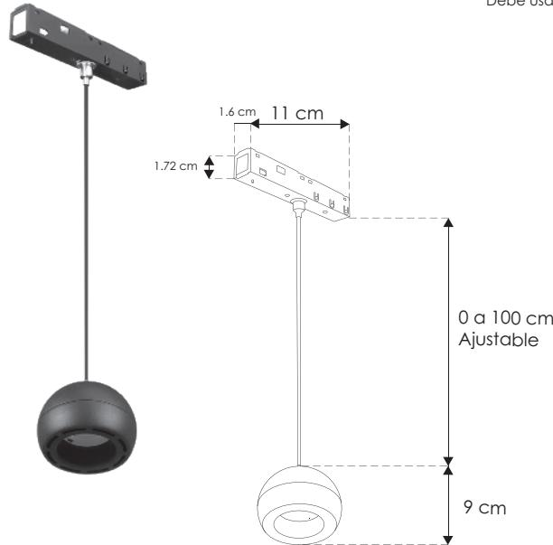
NOTA: Compatible con rieles magnéticos modelos ILUTMAG2624SS, ILUTMAG2651SS, ILUTMAG6246EMP e ILUTMAG6246ETRIM.
